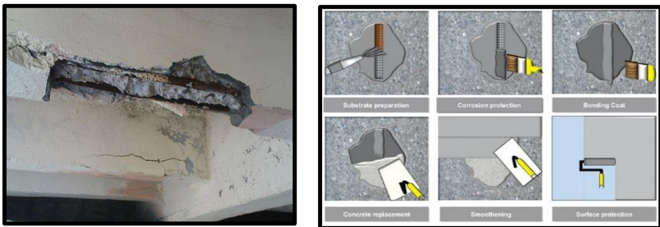
Figure 45 Corrosion Mechanism, prevention & repair measure of RCC structure
